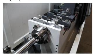
The IMSA deep hole drilling machines of the MFT Series are dedicated to cylindrical workpieces that have to be drilled on their rotation axis.
