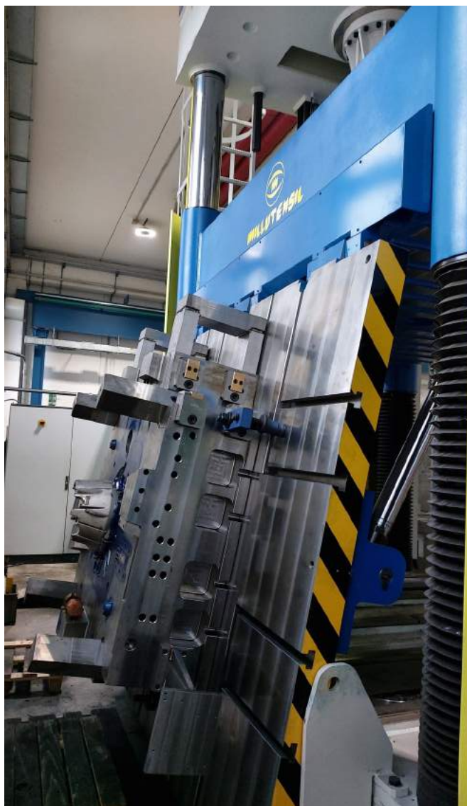
A tryout press is present in the work shop
