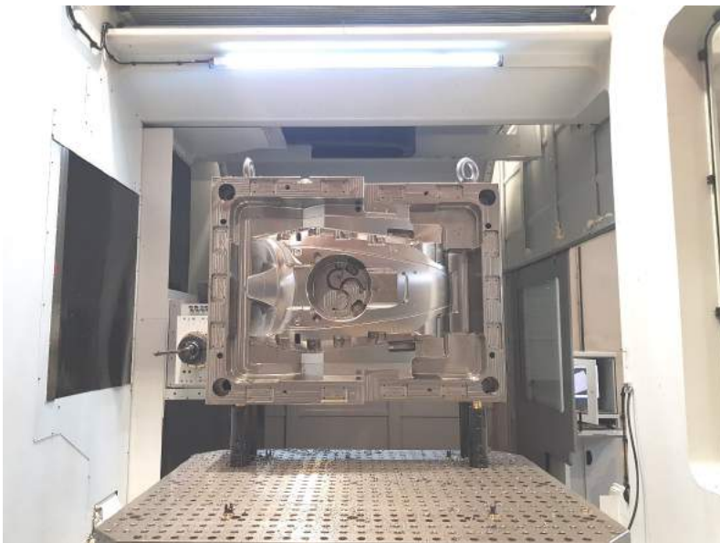
Mould mounted on the MF 1450BB drilling machine
