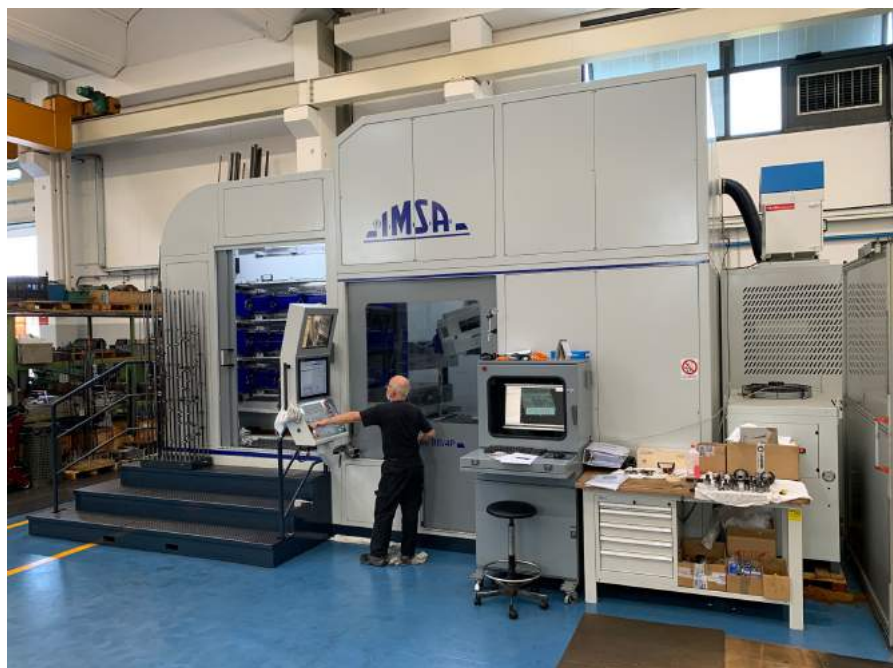
||| The IMSA MF1300/4P EVO deep hole drilling center installed in the tooling shop of R.S. Meccanica.
