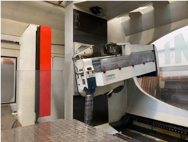
III I.M.S.A. deep drilling centers are equipped with separate spindles for deep drilling and milling with fully automatic switching.
