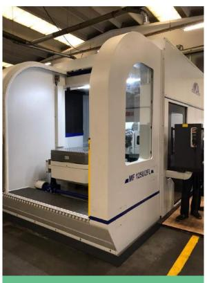
III The deep drilling and milling machine MF1250/2FL by I.M.S.A. located at Mould Solutions.
