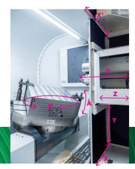
MF1000/2C is available in two versions: for workpieces up to 2 tonnes or for workpieces up to 4 tonnes. Learn more on page 8.
