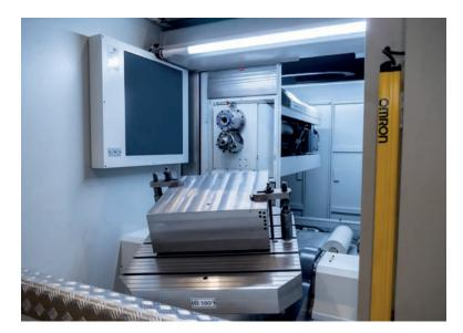
Version "2 tonnes" with rotary/tilting table
