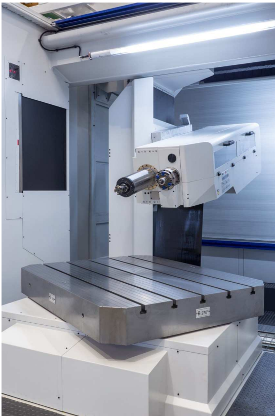
||| Compound angle machining is achieved by rotating the table and tilting the ram.
