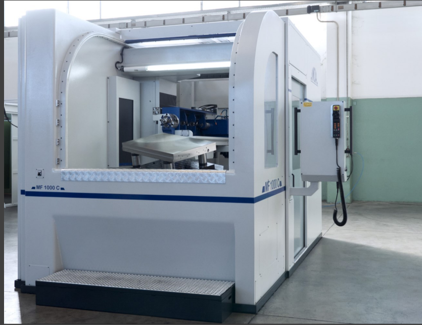
Deep drilling/milling machine for mold inserts, small molds and for other workpieces; the IMSA MF1000C is a compact machine.
