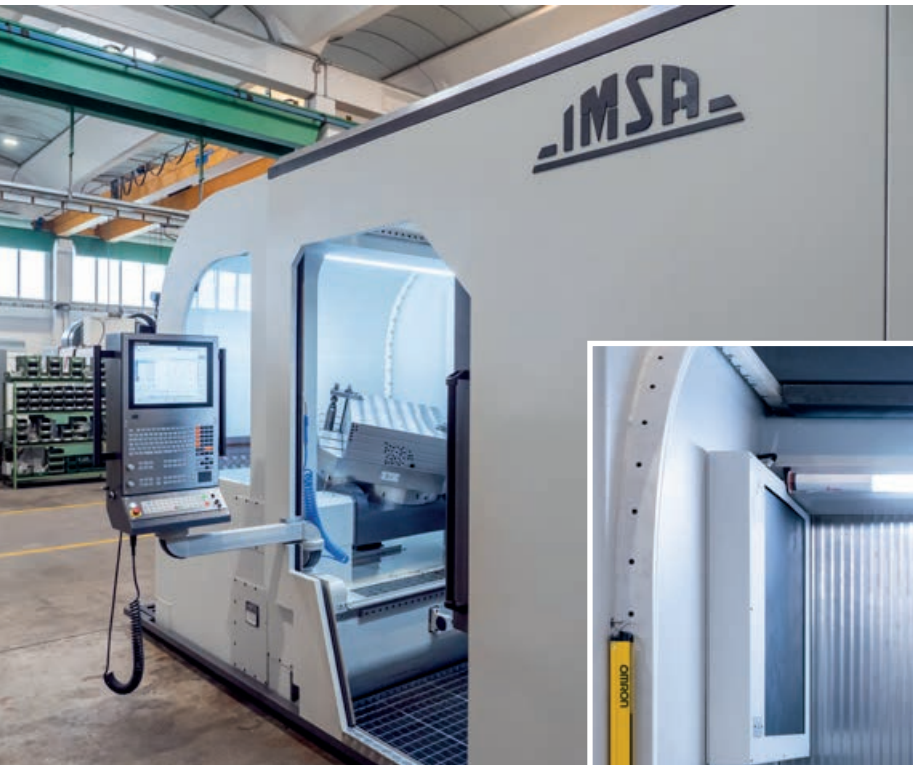
The MF1000/2C machine can be equipped with a fixed or rotary table or with a roto-tilt table, as shown in the picture
